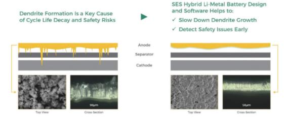
In addition to the electrolyte, our Li-Metal battery cells use a proprietary anode coating that helps provide another layer of protection against dendrites and makes lithium plating denser during charging, as well as an advanced AI-powered algorithm to accurately monitor the state-of-health of the battery cells and detect any impending dendrite-related (or other) safety issues much earlier.
