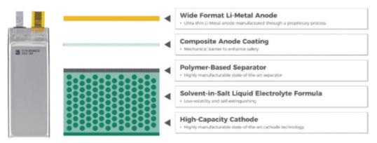
...Combined in a Proprietary Cell Design for Optimized Performance and Safety
