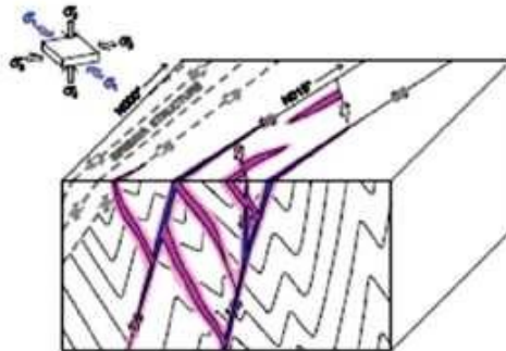
(2C) During D3, along with the breccia injections, multiphase hydrothermal alteration of wallrock.
