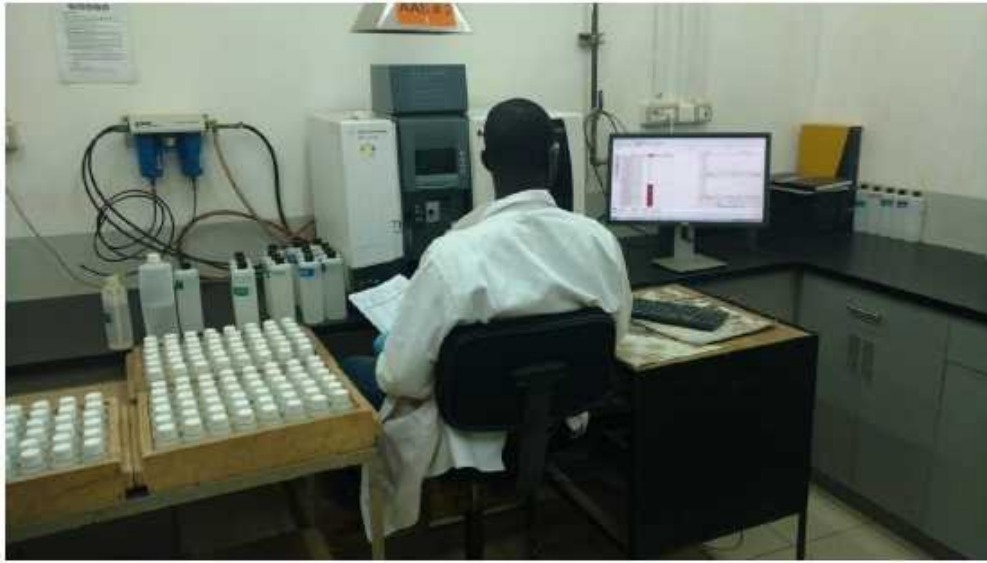
Figure 11 .5: Spectrometry of Leach Solution
