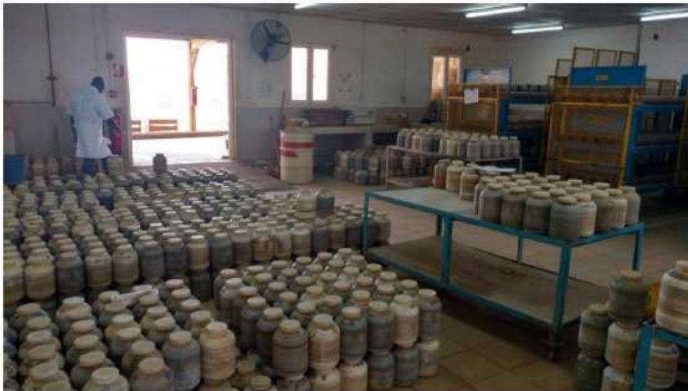
Figure 11.4: Leachwell Samples During the Leaching Process. Note Batches of 24 on the Racks
