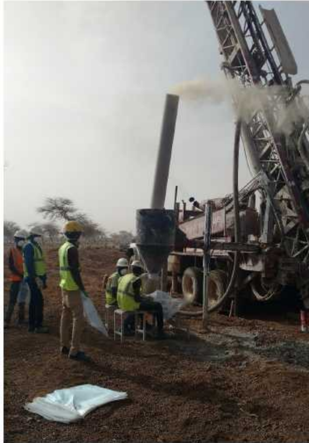
Figure 10.4: Reverse Circulation Drilling at Gossey – March 2018
