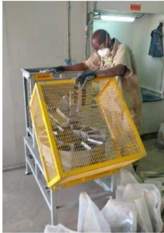
Figure 11.4: Leachwell Samples During the Leaching Process. Note Batches of 24 on the Racks
