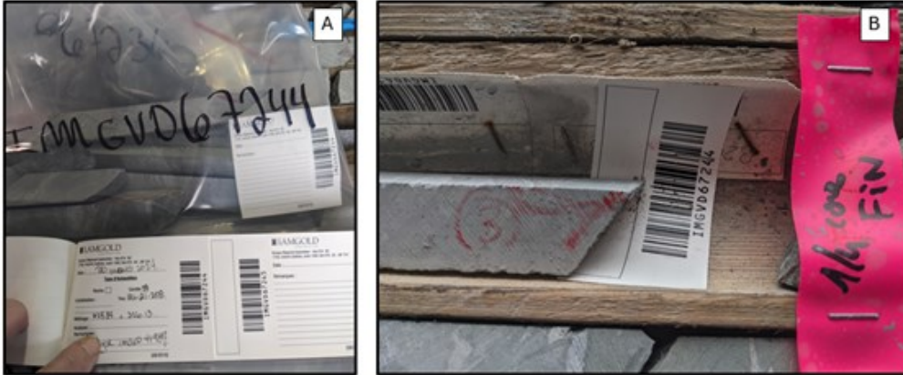
Figure 12.4 - Photograph of core resampled by InnovExplo: (A) method for sample identification; (B) remaining quarter-core witness samples. Hole ML-21-258.
