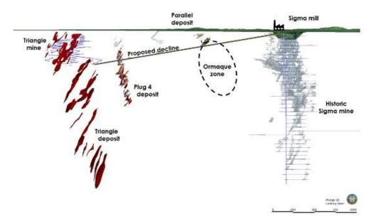
Figure 1: Section view of proposed decline from the Sigma mill to the Triangle mine
