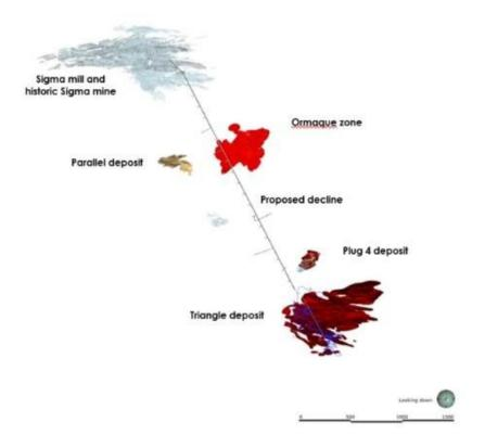
Figure 2: Plan view of proposed decline from the Sigma mill to the Triangle mine
