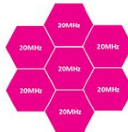
Figure 7: Cell Split to 7 Cells Covering Same Area (7X improvement in capacity)
