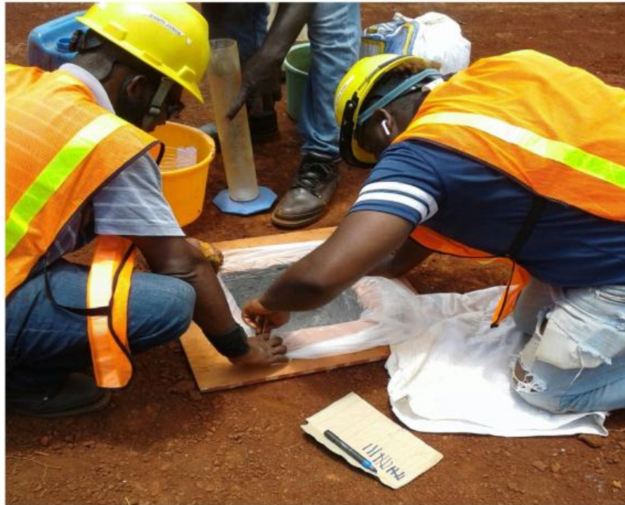
Figure 7-4 In-situ Density Testing
