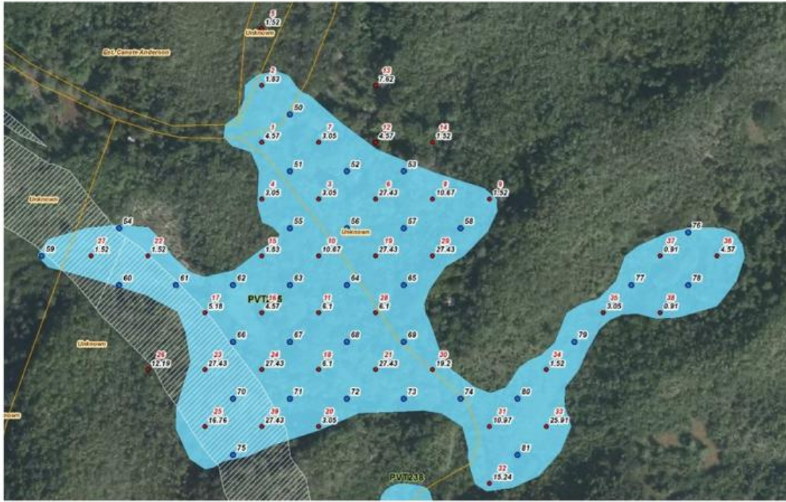
Figure 7-1 PVT Pit 235 JBI Exploration Holes for Resource Drilling
